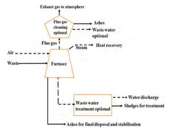
Fig. 3. Simplified flow scheme of Incinerator.
